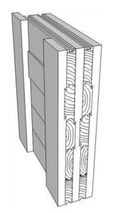
Figure 6. Interlocking CLT. © Cocis
